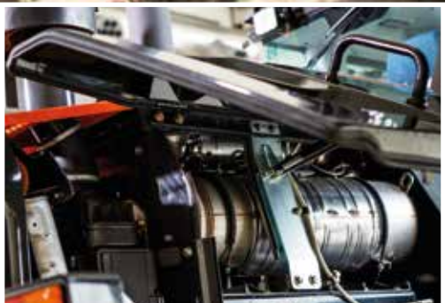
NO DPF SCR system reduces emissions.
