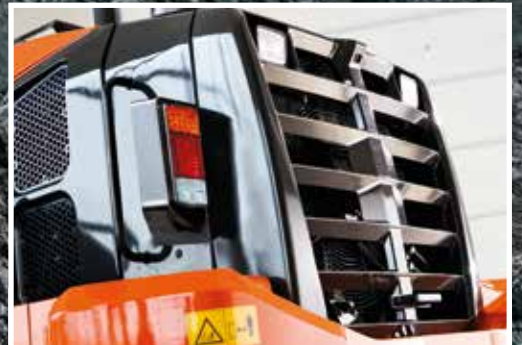
Optional wide fin radiators enhance durability.
