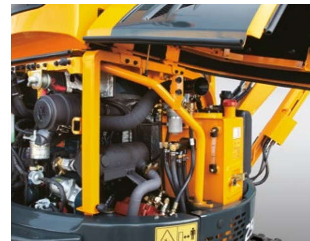
Engine hood/cover Wide opening doors, covers and hoods provide easy access for servicing tasks.
