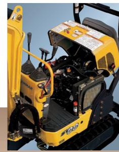
Large opening engine hood and is covered by a protective shield. removable side frame cover provide easy accessibility for maintenance.
